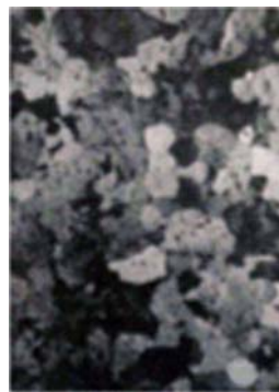
Sample No.2 Annealing temperature 880 °C, 5 min. period
