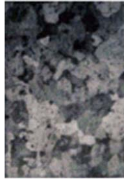
Sample No.3 Annealing temperature 880 °C, 15 min. period
